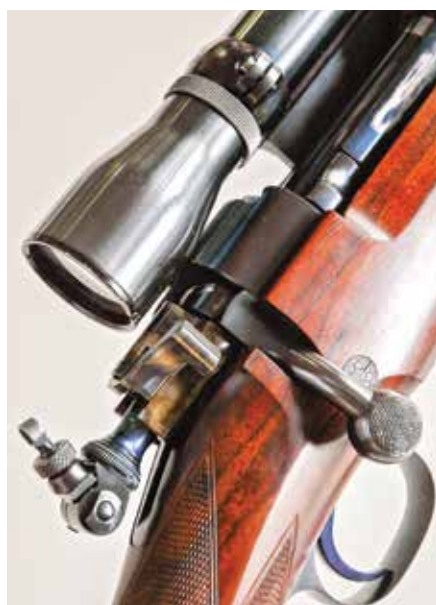
Long eye relief and short eyepieces were once the rule. On this Heineke Springfield, sight and scope could both be used without moving the head on the stock.
