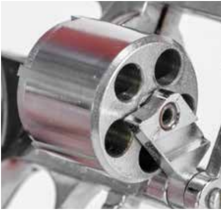
The cylinder is held in place with what appears to be a brass rivet, through which an easily lost spring-loaded pin is inserted. The pin (inset) also serves as the extractor.
