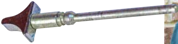
The cylinder is held in place with what appears to be a brass rivet, through which an easily lost spring-loaded pin is inserted. The pin (inset) also serves as the extractor.
