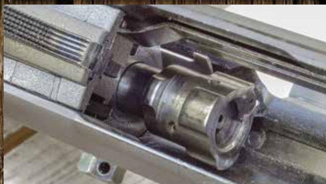
The Kronos Rifle uses a three-lugged rotation bolt head like those in Pietta shotguns.
