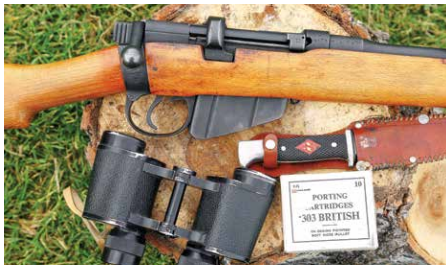
The Lee-Enfield No. 1 Mk III, designed before 1900, is still unsurpassed in speed of reloading. The bolt knob is above the shooting hand and it has a short, easy bolt lift and throw.
