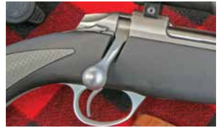
A long bolt handle ideally located, short (70 degrees) bolt lift, short bolt throw, and superb workmanship on Dave's favorite rifle, his little Sako Finnlight .243.
