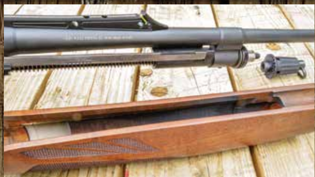
The short-stroke gas system of the Pietta is very similar to the Browning BAR.
