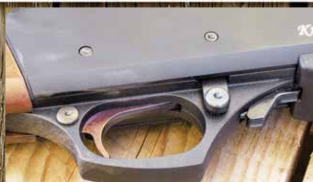
The push button safety, bolt hold-open and magazine release are clustered around the trigger guard.
