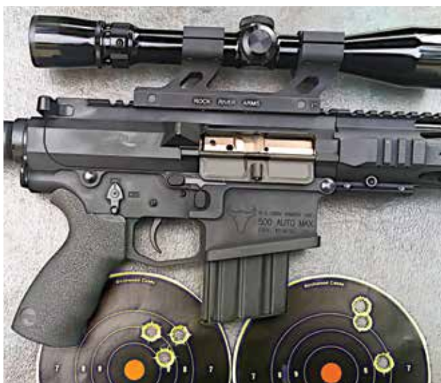
Typical accuracy from the AR500 Auto Max pistol at 100 yards. Groups ranged from 0.9 to 2" as these groups demonstrate. Great accuracy for such a powerful pistol.
