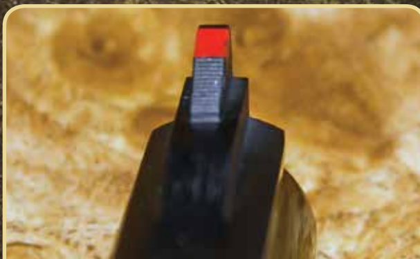
A major factor in successful handgun shooting is seeing the front sight. The M25's orange insert helps in the diminished light conditions predators favor.
