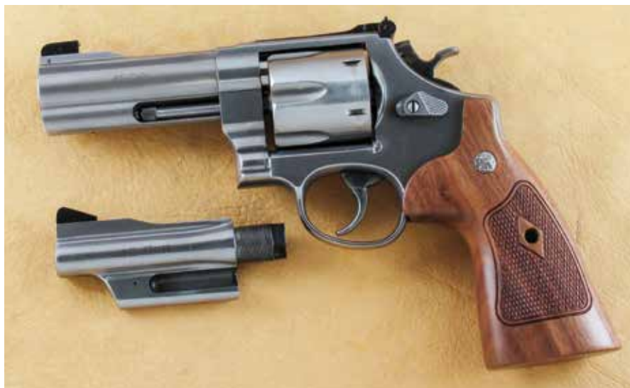
The barrel of this S&W Mountain Gun was replaced with a heavy underlug version after a defect was discovered while trying to decide why it wouldn't shoot straight.
