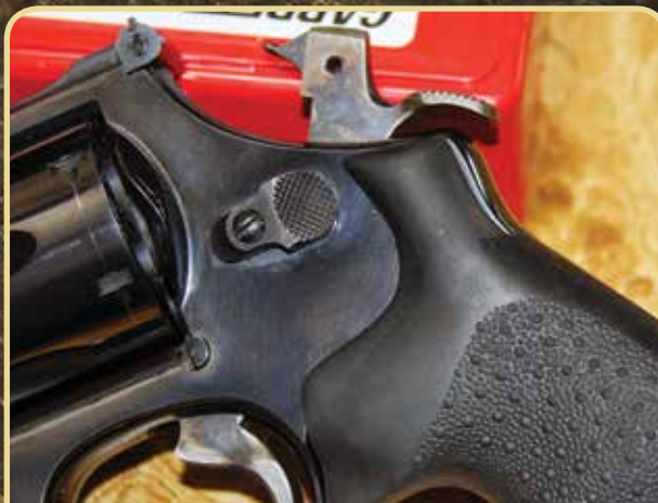
Hammer-mounted firing pin and absence of "key hole" in the frame reveal some of the old school features of the Model 25, while the stippled Hogue grips facilitate shot-to-shot recovery.
