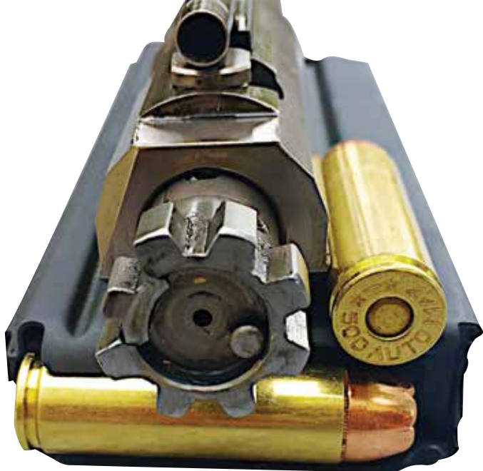
The bolt-face was opened up to accept the 500 Auto Max head. Extractor and ejector were strategically placed for optimal performance.
