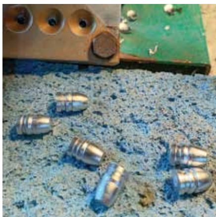
The Lee 6-cavity mold makes a pile of bullets in a hurry. Here's six freshly cast bullets straight from the mold.
