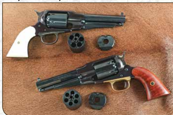
This Richards Conversion (above, top) and the Richards-Mason Conversion are both chambered in .38 Long Colt/.38 Special. These 5-1/2" 1858 Remington percussion pistols (below) in .44 and .36 are easily changed into Cartridge Conversions using conversion cylinders from Taylor's & Co.
