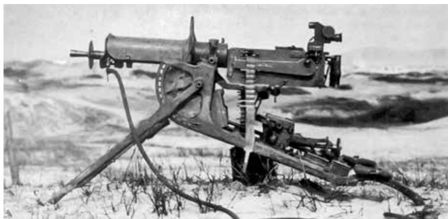
The MG08 Maxim machinegun with its massive sled mount weighed some 152 lbs. It could only be used from fixed positions as a result. Public domain photo: Wikipedia
