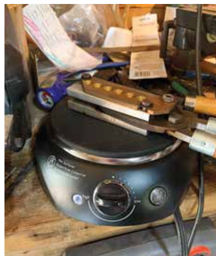
Pre-heating your mold allows perfect bullets to be cast on the first cycle.
