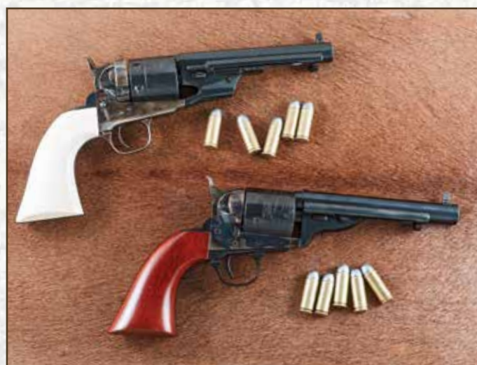
This Richards Conversion (above, top) and the Richards-Mason Conversion are both chambered in .38 Long Colt/.38 Special. These 5-1/2" 1858 Remington percussion pistols (below) in .44 and .36 are easily changed into Cartridge Conversions using conversion cylinders from Taylor's & Co.
