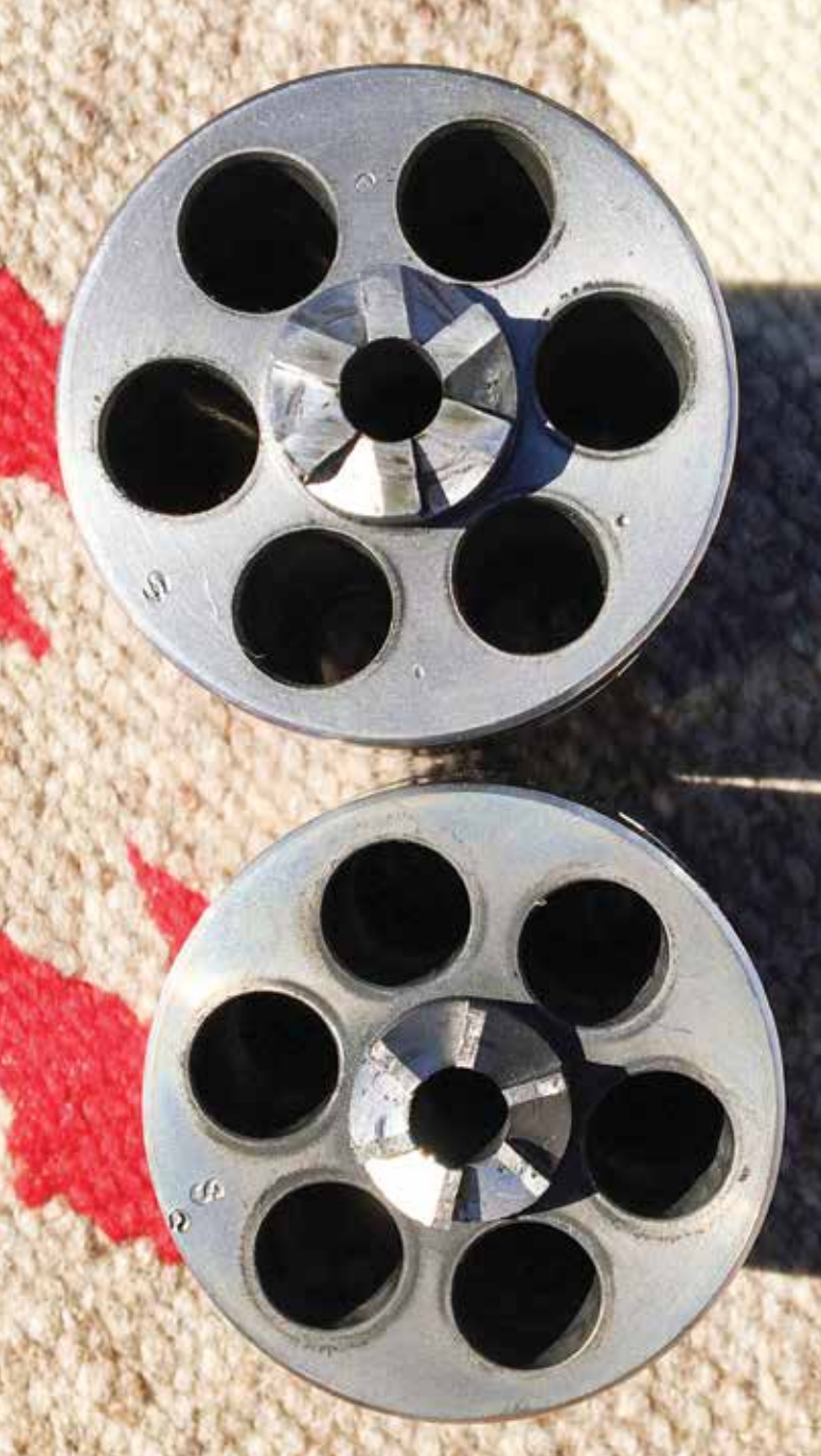
To slim down the “New Model” while maintaining Vaquero’s legendary strength, they moved the chambers inward. Original (top cylinder), New (bottom cylinder). Even with fixed open sights and aging eyesight, the Vaquero performs well at 25 feet (below).
