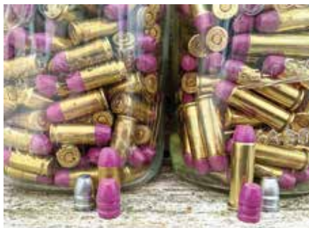
Here's a close up of Lee's 358-125 RF bullet cast by Tank. They are an exceptional bullet for .38/.357 and 9mm fodder.
