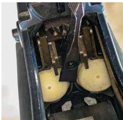
A three-position magazine cut-off switch rests between the tubes, allowing you to easily choose between loads such as slug and buck. No "select slug" drills here!
