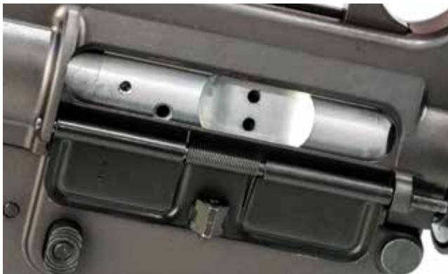
The bolt carrier is hard chrome plated like the originals and is locked rearward by a trigger inside the carry handle.
