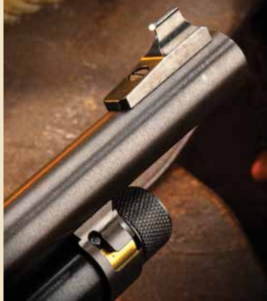
The ramp front sight offers a traditional-style white bead. Below the barrel rests the knurled tube-magazine loading knob for loading and unloading.
