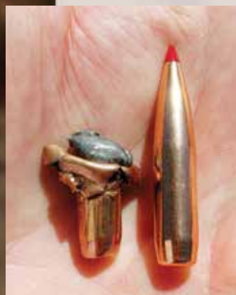
Hornady's 143-gr. ELD-X bullet exhibited outstanding performance with a retained weight of 105 grains.
