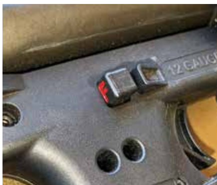
The safety is standard cross-bolt type. Push to the right to make a big noise!
