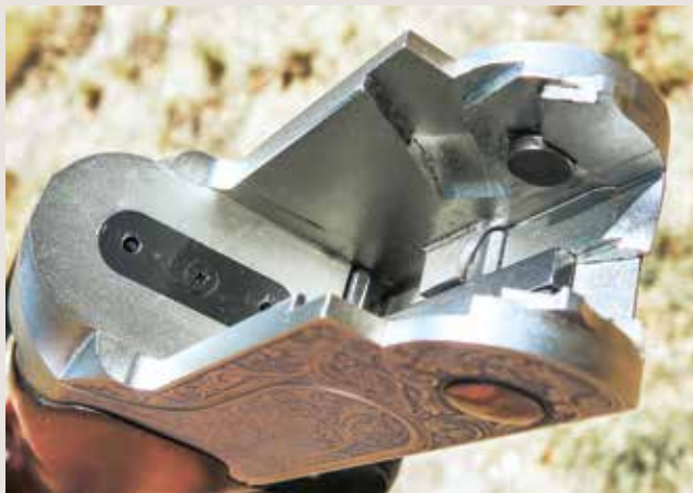
To control weight, the receiver is machined from aluminum with steel trunnions and a steel-reinforced standing breech face.
