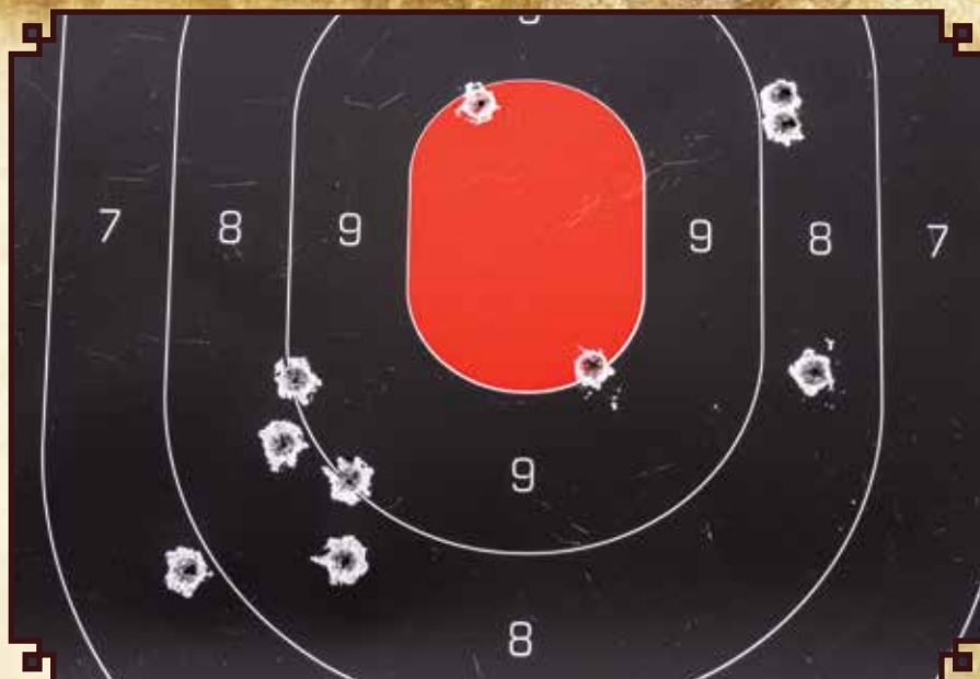
The low 2½" group is Duke's handloads, followed by a group with Winchester's factory loads (after rear sight was raised) of 4½" due to undersize bullets.
