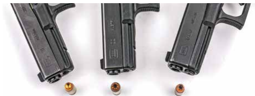
The .40 GLOCK 22 (center) can be turned into a G31 .357 (left) with just a barrel change and can duplicate a G17 (right) with a 9mm barrel, magazine and recoil spring assembly.
