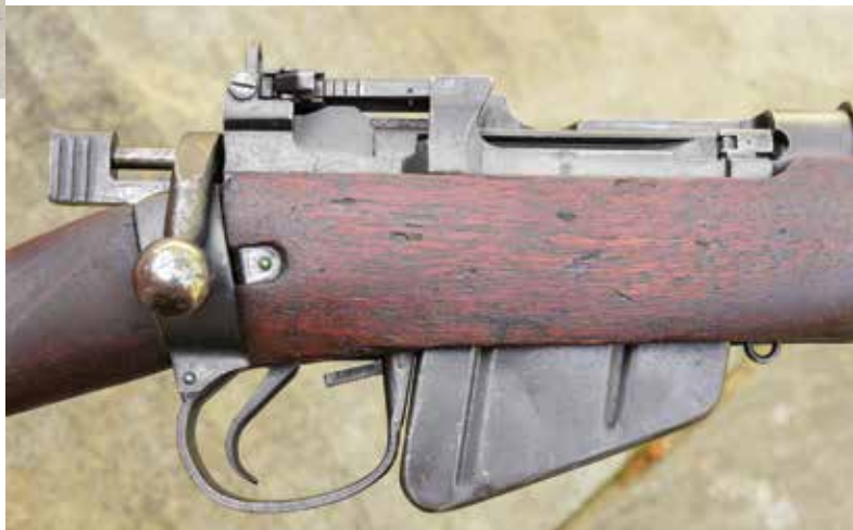
The bolt handle on the No. 4 is located behind the trigger guard for fast operation.
