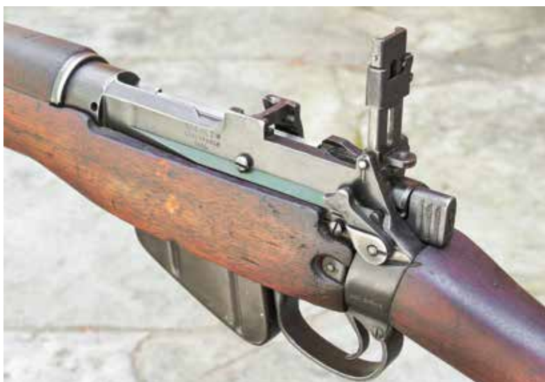
A simplified sheet metal rear sight and square (instead of rounded) metal surfaces made the No. 4 easier to manufacture. Note the Long Branch markings on the side.
