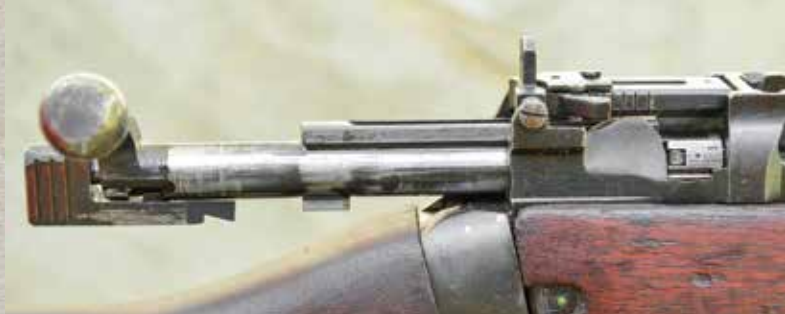
The rear bolt-locking lugs were not as strong or precise as front-mounted Mauser-style lugs but they were good enough.
