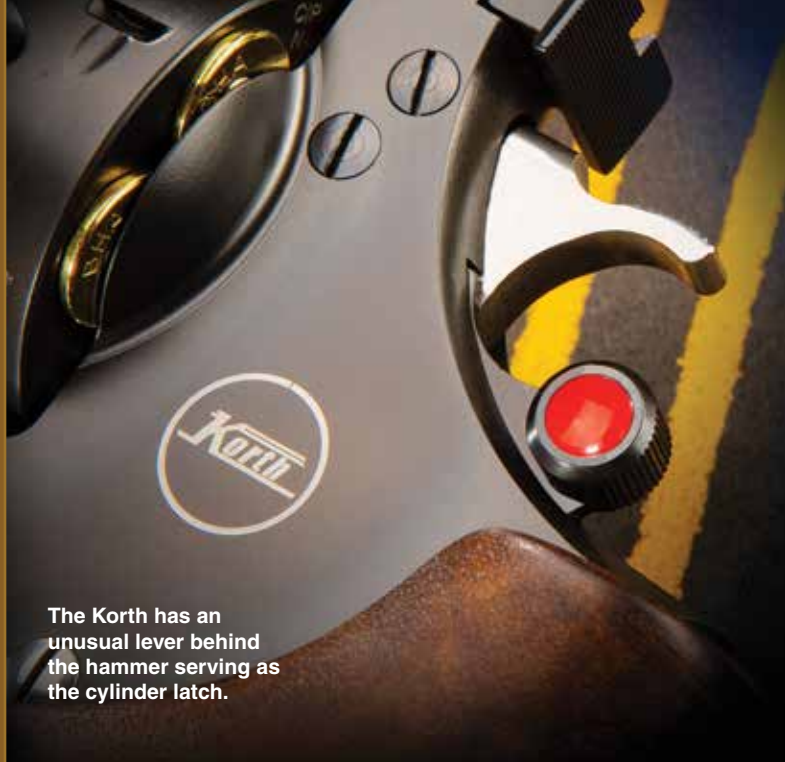
The cylinder offers plenty of room for fast loading and unloading. Press a button on the right side of the frame and the cylinder removes for cleaning.
