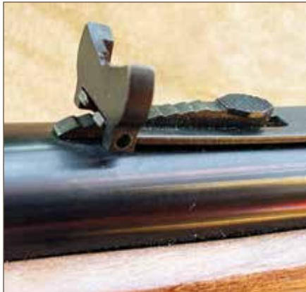
A folding, adjustable semi-Buckhorn rear sight is standard. Denny replaced it with a Skinner Sights aperture sight and used a Skinner blank to fill the empty dovetail.
