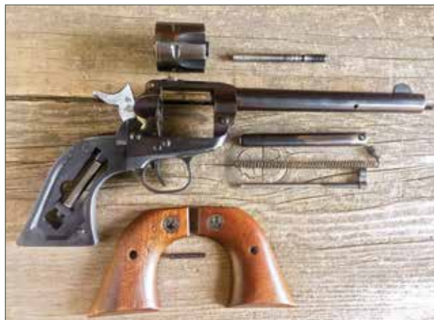
As issued in 1962: walnut grips with post-Alexander Sturm eagle medallion, frame/barrel assembly with coil mainspring and contoured loading gate (this replaced the original flat gate), .22 WMR cylinder and base pin, ejector rod, spring and housing.
