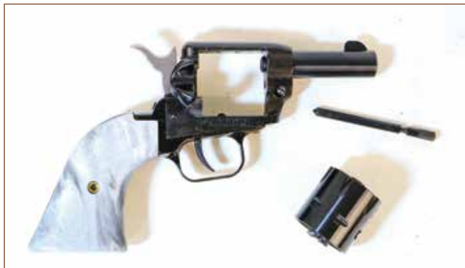
To remove empty cases, just set the hammer to half cock, open the loading gate and poke them out from the front with the included tool. If you lose it, a length of coat hanger wire also works fine! Disassembly of the Heritage Firearms Barkeep (below) is a snap without tools.
