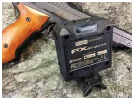
Tom shoots the frangible Dust Devils at standard steel plates, in his garage. This FX Pocket Doppler Radar chronograph (below) isn’t much larger than a deck of cards.
