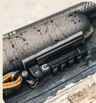
Mark added Caldwell's PIC Rail Adaptor Plate to the sling stud, giving the rifle a Picatinny rail mounting point for a bi-pod and a sling attachment.
