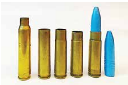
The simple steps of converting 5.56/.223 brass to 300 BLK. Looks like fun, eh?
