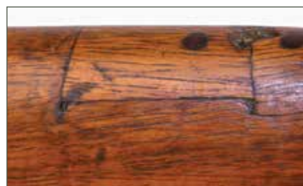
The stock of this German Spandau Gew 98 rifle was damaged near the comb. Some long-dead artisan very skillfully excised the broken bit and made a plug to repair it.
