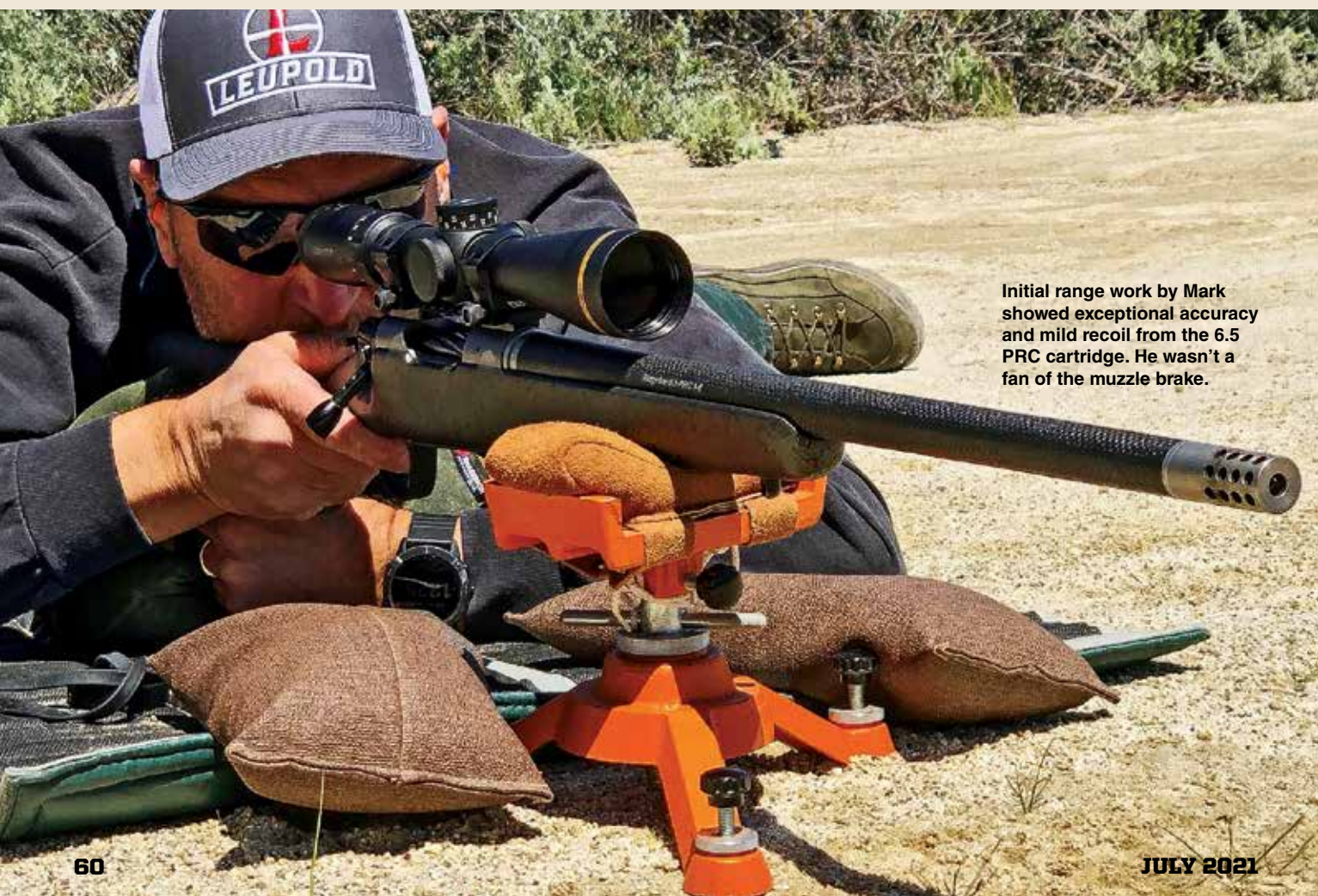
The lightweight titanium receiver, carbon fiber-wrapped barrel and carbon fiber stock give the Ridgeline Titanium its nimble feel and agility.
