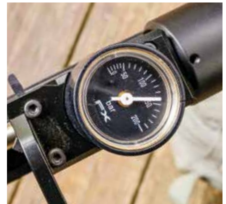
The secondary manometer helps you control regulator pressure adjustment — and is also customizable.
