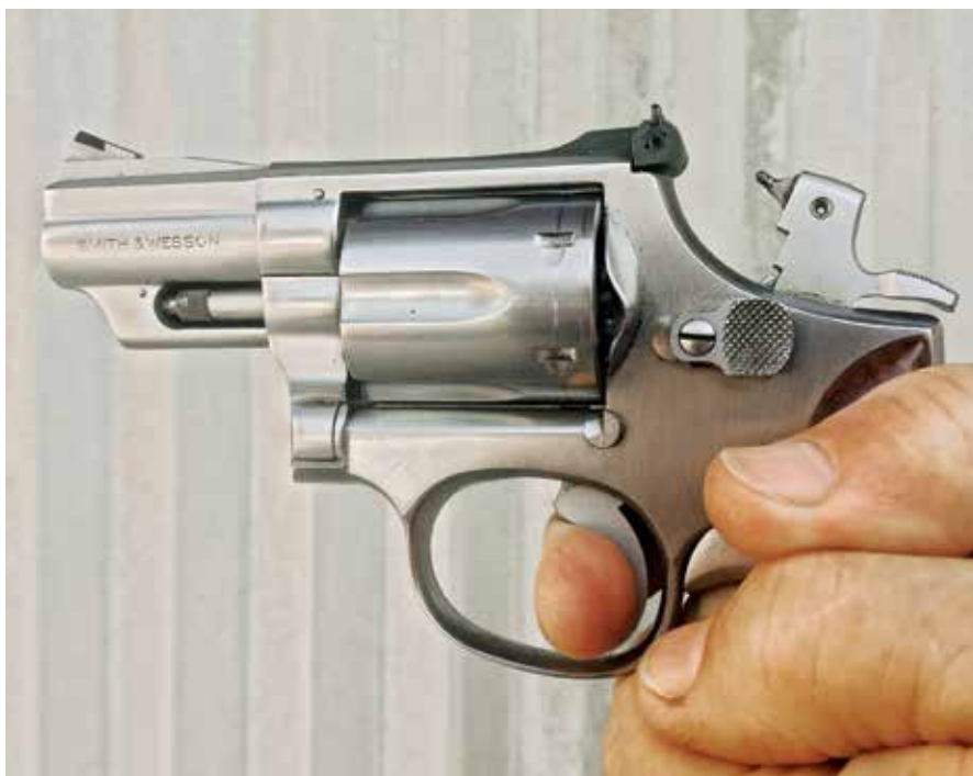
M66 "Dash-1" features include (above) a pinned barrel, hammer-mounted firing pin and recessed charge holes (below).
