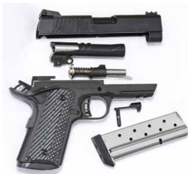
TAC Ultra CS field-stripped for cleaning. A bent paper clip keeps the spring/guide assembly together for removal from the slide.
