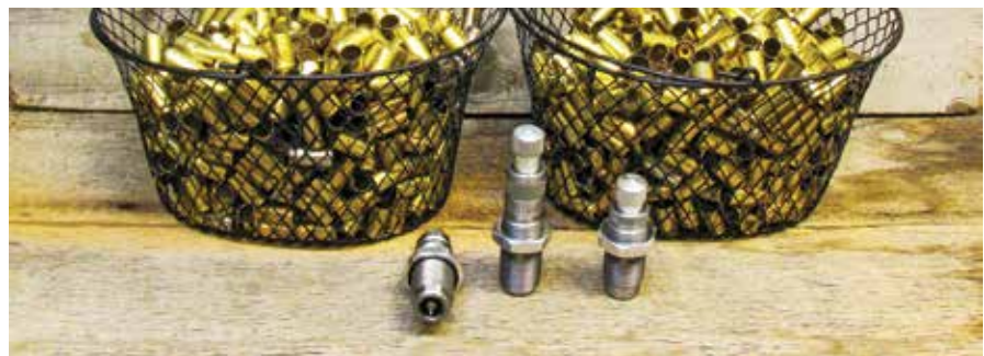
A worthy project during the lockdown — 1,000 .45 ACP cases along with Lee Under-sized Carbide Sizing die, Universal Expander and Factory Crimp Die.
