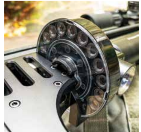
The magazine (above) is fantastic, one of the most reliable designs Tom has tested. The power wheel settings are unique (left) and offers 12 preset adjustments.
