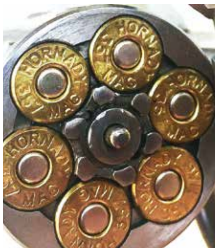
M66 "Dash-1" features include (above) a pinned barrel, hammer-mounted firing pin and recessed charge holes (below).
