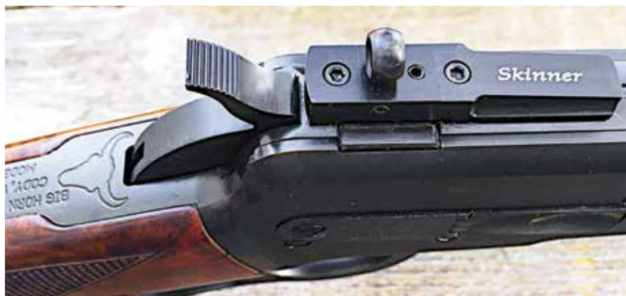
Factory-supplied Skinner Sights (above) peep sights on the BHA Model 90 allows for fast, accurate shooting. Tank loves them! The bare bones basic TCA Encore with a 20" Katahdin barrel is a pure utilitarian carbine (below), while the beautiful BHA Model 90 exemplifies what a levergun should be.
