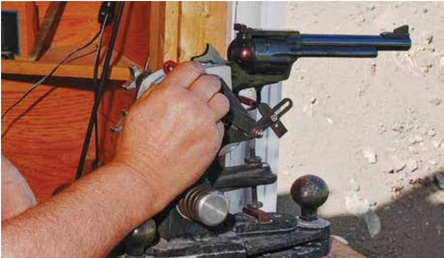
Duke test firing his Old Model .44 Magnum from Ransom Pistol Machine Rest.
