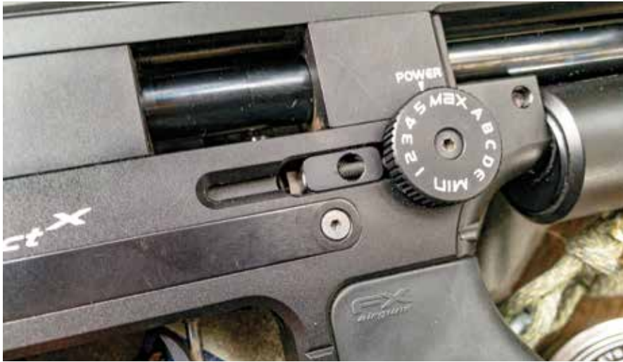
The magazine (above) is fantastic, one of the most reliable designs Tom has tested. The power wheel settings are unique (left) and offers 12 preset adjustments.
