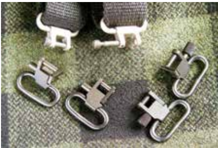
Sling swivels come in all shapes, sizes and prices. Inexpensive versions often fail after a short time so bargain-basement swivels are often not the deal they may seem.
