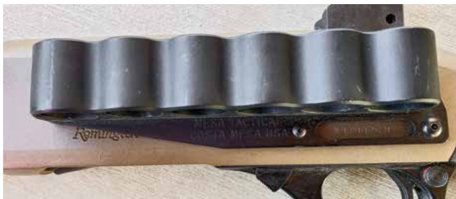
A receiver-mounted shell carrier (above) is more useful than a butt cuff — you don’t have to alter your firing grip or lose sight of danger.
