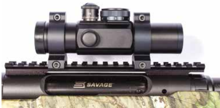
On Mark's test gun an UltraDot MatchDot II was mounted on the one-piece rail.
