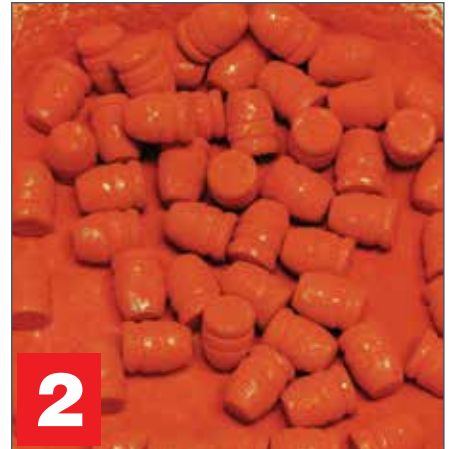
Step two: Powder is added, the lid shut and the affair given a two-minute shake until everything is thoroughly coated.
