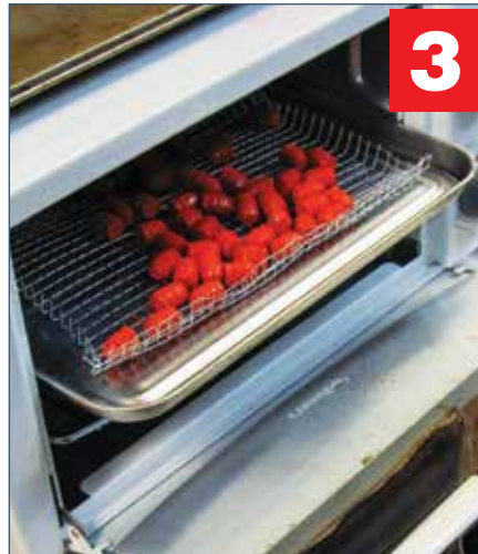
Step three: The bullets go into the toaster oven inside John's homemade 1/4" mesh basket. Don't get too hot or the bullets might melt!
