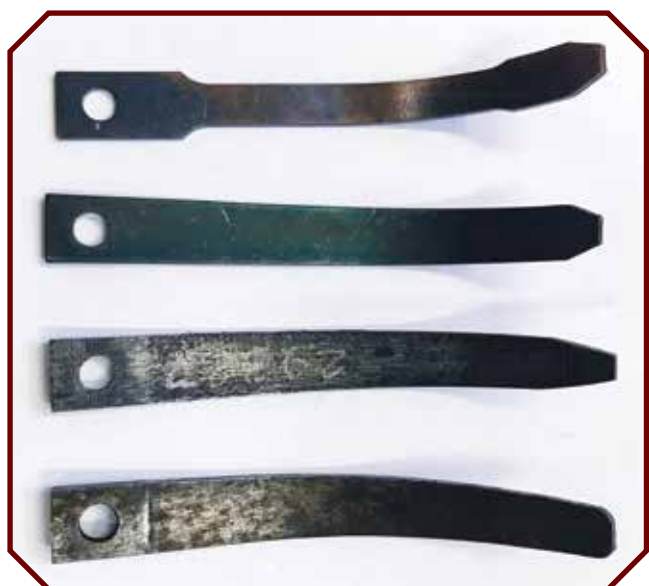
Original Colt SAA mainsprings (bottom) were quite strong. By the end of the First Generation run, the thickness had diminished. Third Generation Colt SAAs sport a much thinner and narrower mainspring. Photo: Peacemaker Specialists
