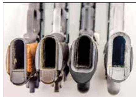
Mag well progression on some of Mas' Colt 1911s. Above from left: Stock GI style, beveled, small funnel, wider funnel.
