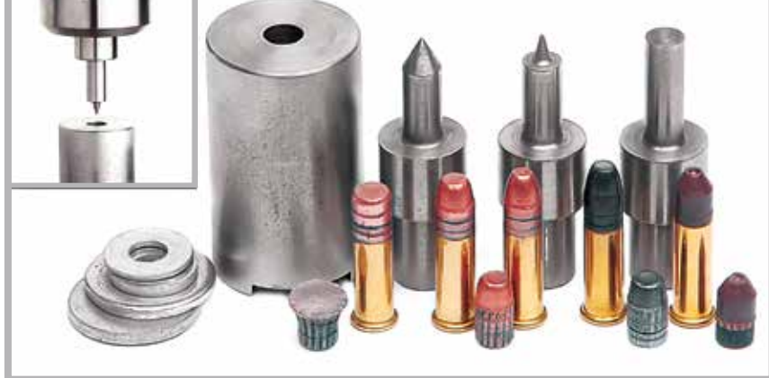
The Li'l Gizzy hollow- and flat-pointing tool set comes with the die and rams to make small and large HPs and FPs. Roger used a drill press (not running), but you can also use a soft-faced hammer.
