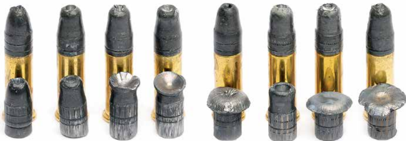
Modified Roundnoses, left to right: CCI Quiet 22 RN, 40-grain, Li'l Gizzy small HP plus #0 screwdriver; CCI Quiet 22 RN, 45-grain, Li'l Gizzy small HP; Quiet 22, 45-grain, Li'l Gizzy small HP plus #0 screwdriver; Quiet 22, 45-grain, Li'l Gizzy large HP; Unmodified CCI Suppressor HP, 45-grain; CCI Std. Vel., Li'l Gizzy small HP; CCI Std. Vel., Li'l Gizzy large HP; and CCI Std. Vel., Li'l Gizzy small HP plus #0 screwdriver.
