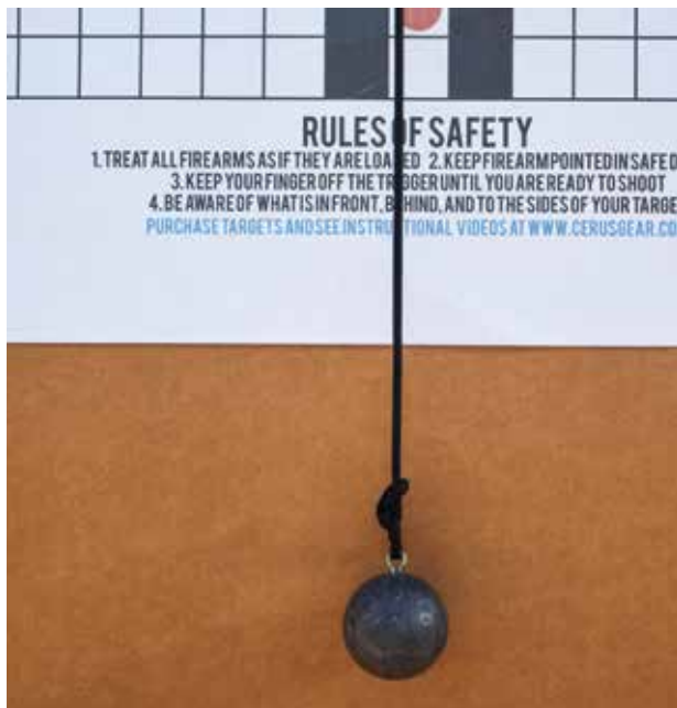
D'Arcy Echols fashioned and now markets this target (above) to help orient scope reticles easily and precisely. A plumb bob in front of this backing board (below) shows "true vertical." The target is aligned with its cord.
