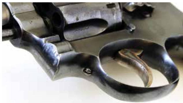
Brutalized screws can be tell-tale signs of softer steels, as much as “Bubba” gunsmithing.
