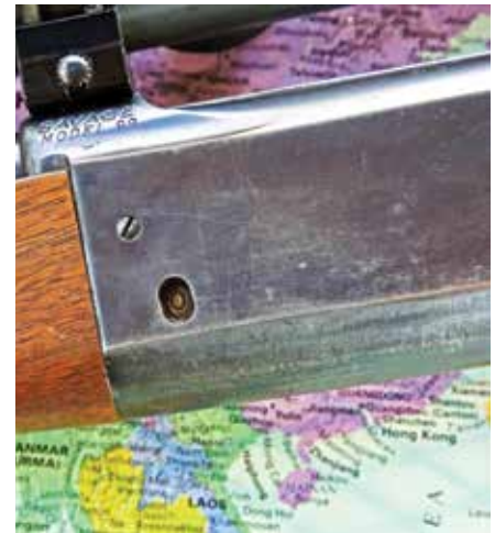
One of Dave's Savage 99s, made in 1954. One of the many fine features of the 99 was the brass rotary magazine. A window in the frame shows the rounds remaining.
