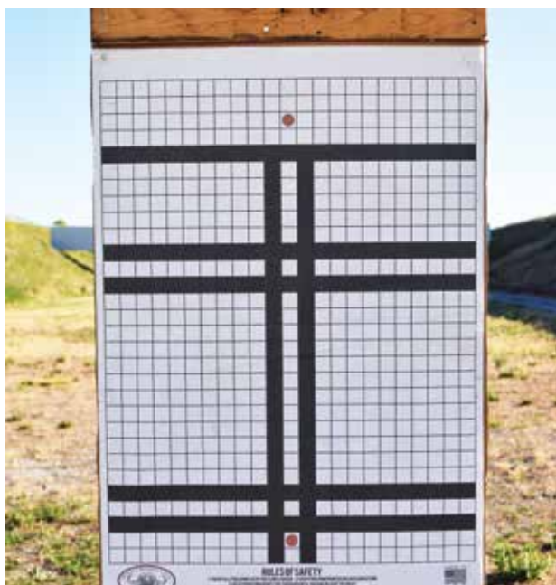
D'Arcy Echols fashioned and now markets this target (above) to help orient scope reticles easily and precisely. A plumb bob in front of this backing board (below) shows "true vertical." The target is aligned with its cord.
