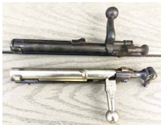
The multi-lug Springfield '03 (top) was stronger than the Krag (bottom). However, the single-lug Krag was plenty strong enough for .30-40 pressures and was as smooth in operation as a bolt action gets!
