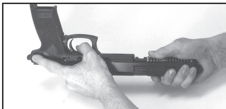
Figure 13 - Correct Position for Holding Slide for Reassembly
