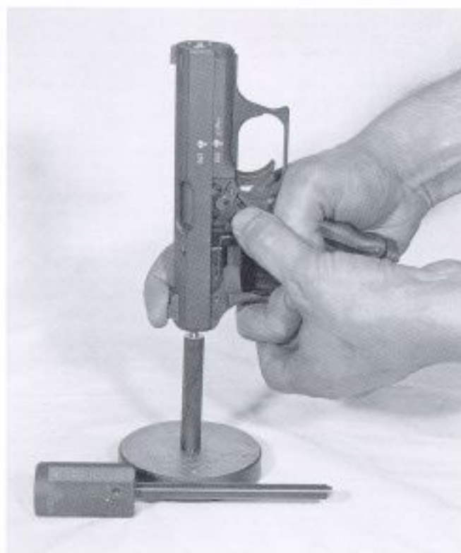
Figure 20. Inspection of firing pin front protrusion.
