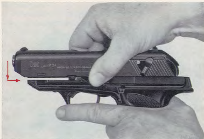
Fig. 13: Place slide on receiver
