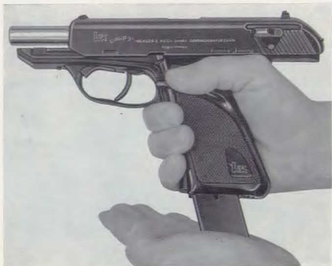
Fig. 7: Reloading the pistol
