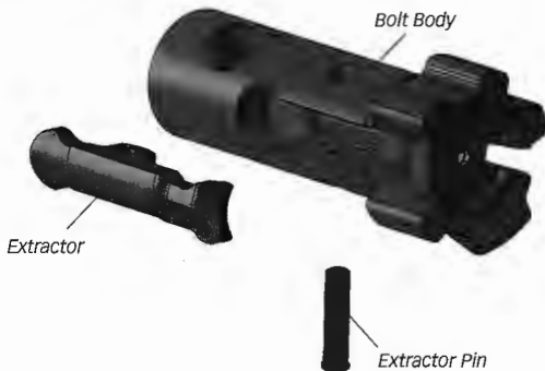
FIG 26 BOLT WITH EXTRACTOR REMOVED
