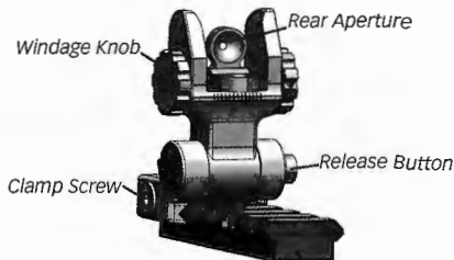
FIG 17 REAR SIGHT WINDAGE ADJUSTMENT
